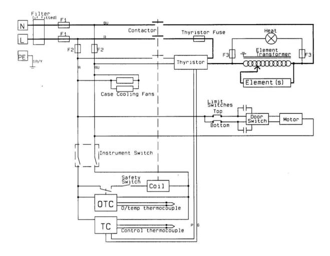
TC temperature programmer OTC overtemperature controller
